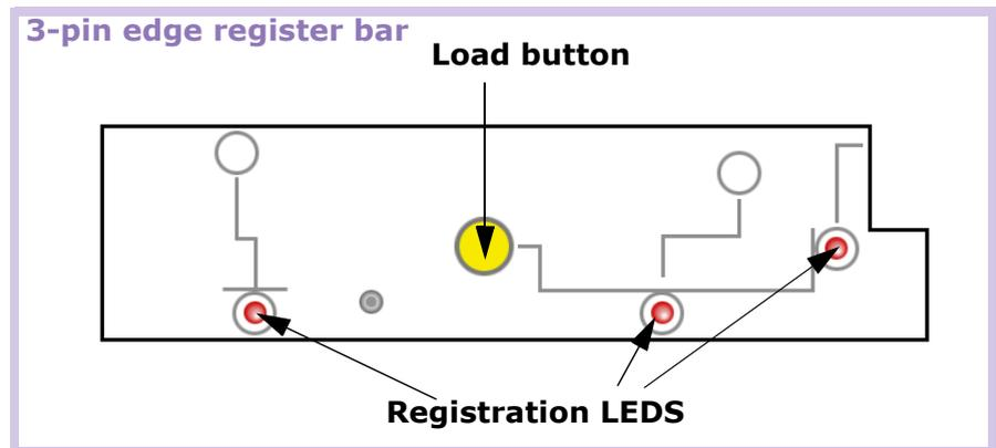
The registration LEDs help you to position the plate correctly. You use the load button to prepare the drum for plate load and to release the vacuum from the plate.
