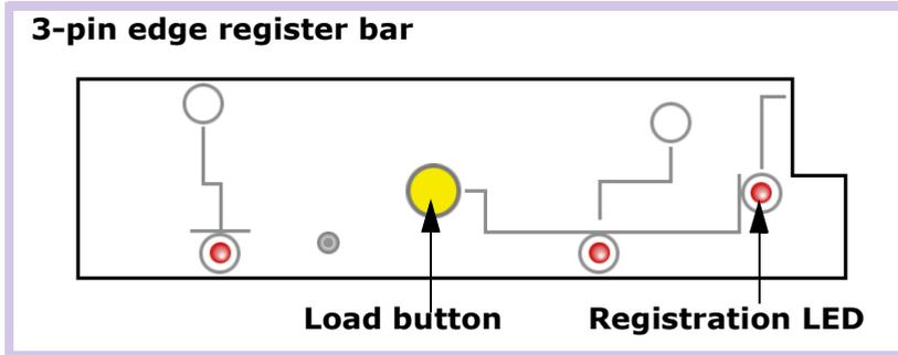
**Note:** If you need to abandon the plate load, press the **Load** button on the register bar to switch off the vacuum pump and to return the register bar to its 'disarmed' state.
